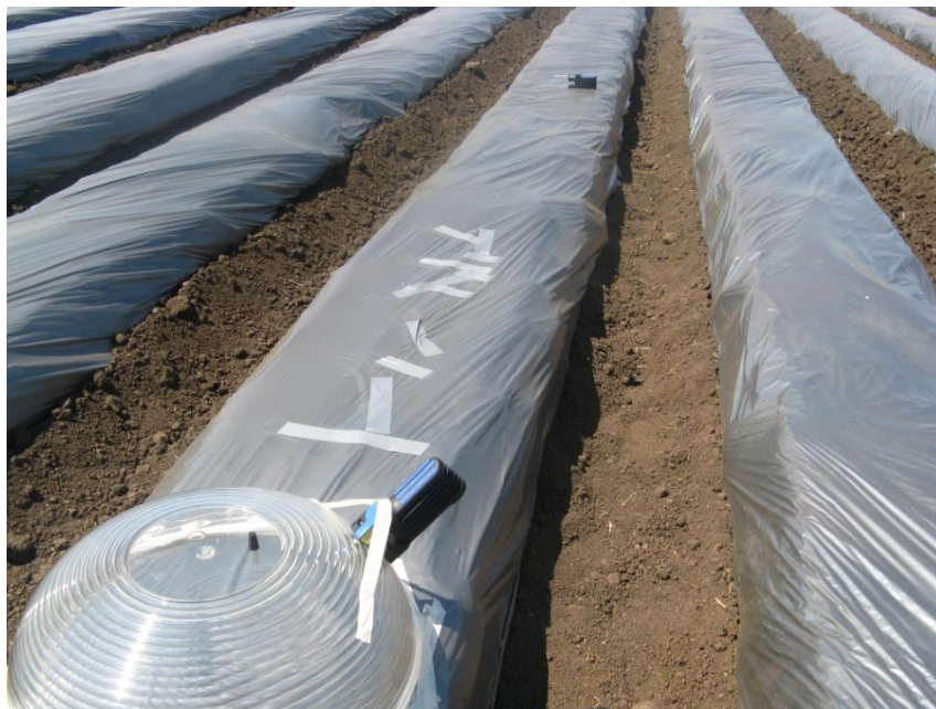
Photo Two: Dräger sampling pump in place on SALAD unit
