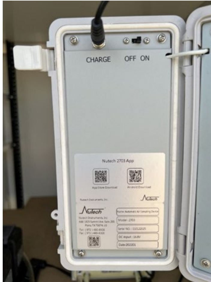
Figure 4: The Nutech 2703 controller is connected to a power source and is turned ON.
