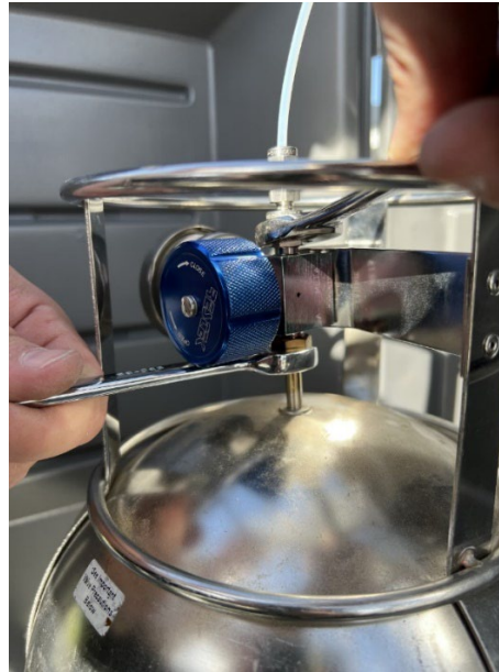
Figure 6. Using a second wrench to hold the bottom fitting in place to prevent damaging the valve stem during tightening process.
