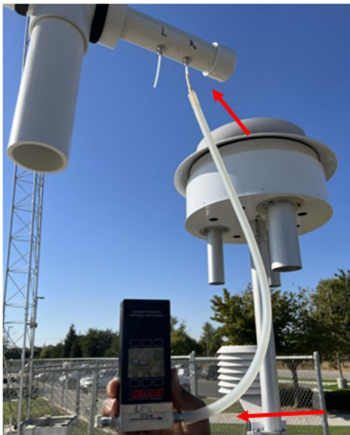
Figure 13: Connection of the ALICAT Scientific low flow meter to take initial and ending flow rates.
