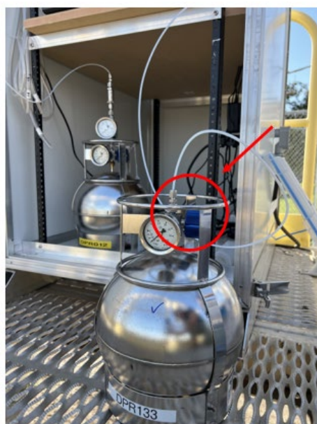
Figure 5: Nutech 2703 tubing connected to a canister.
