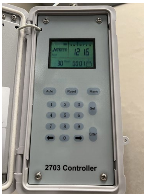
Figure 12: Nutech 2703 controller has started a scheduled sampling event.
