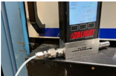
Figure 14. Xonteck output line threaded onto the ALICAT flow meter.
