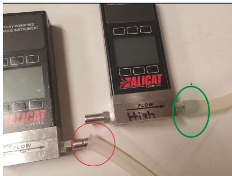
Figure 15. Correct attachment of the tubing to the ALICAT is shown in green circle.
