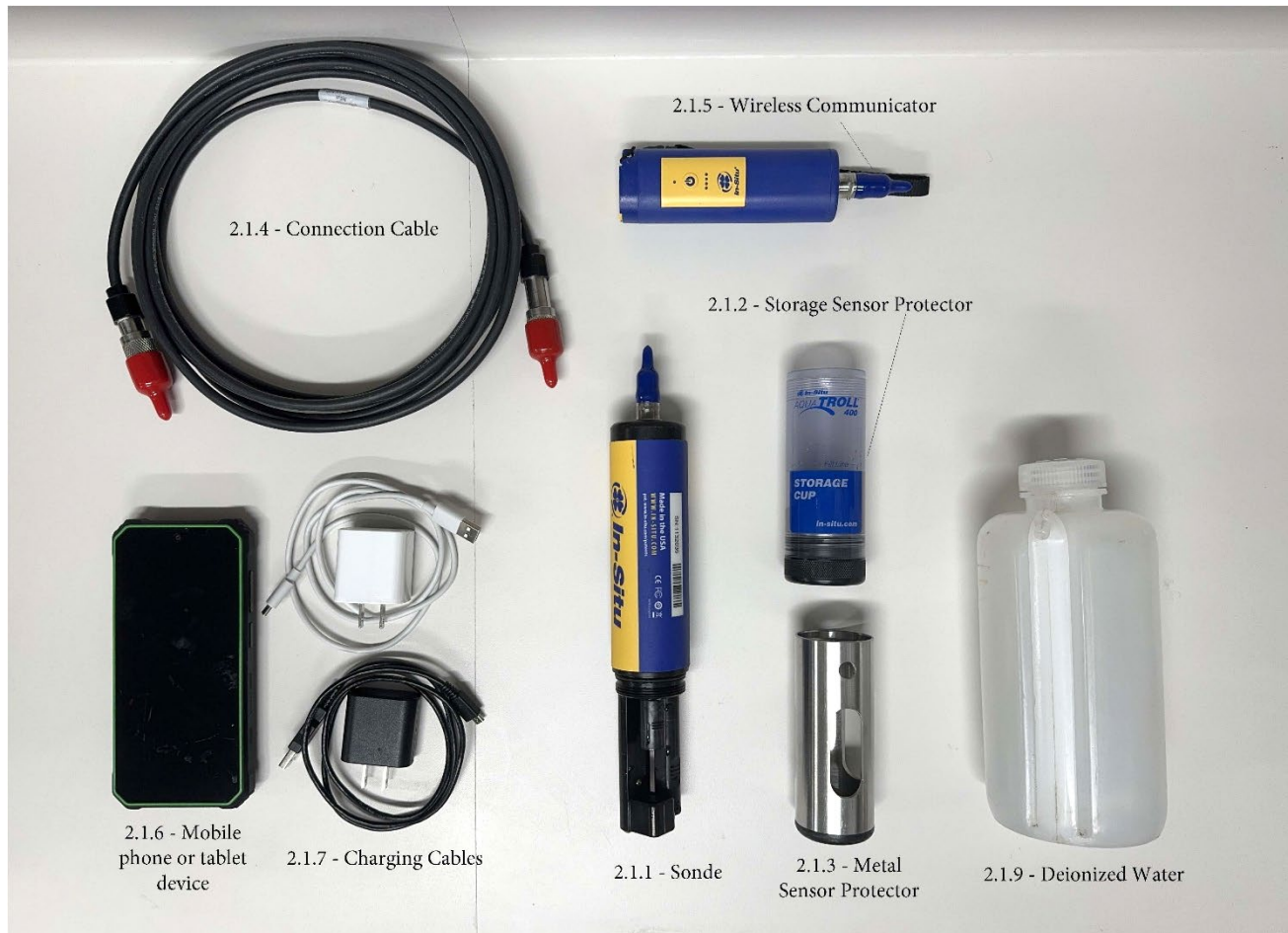
Figure 1. All components needed for the collection of water quality parameters using an Aqua Troll 400 device. Carrying case not pictured.
