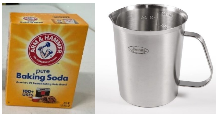
Figure 3: Sodium bicarbonate (for containment and neutralization of spills) and a stainless-steel measuring cup (for sample collection).
