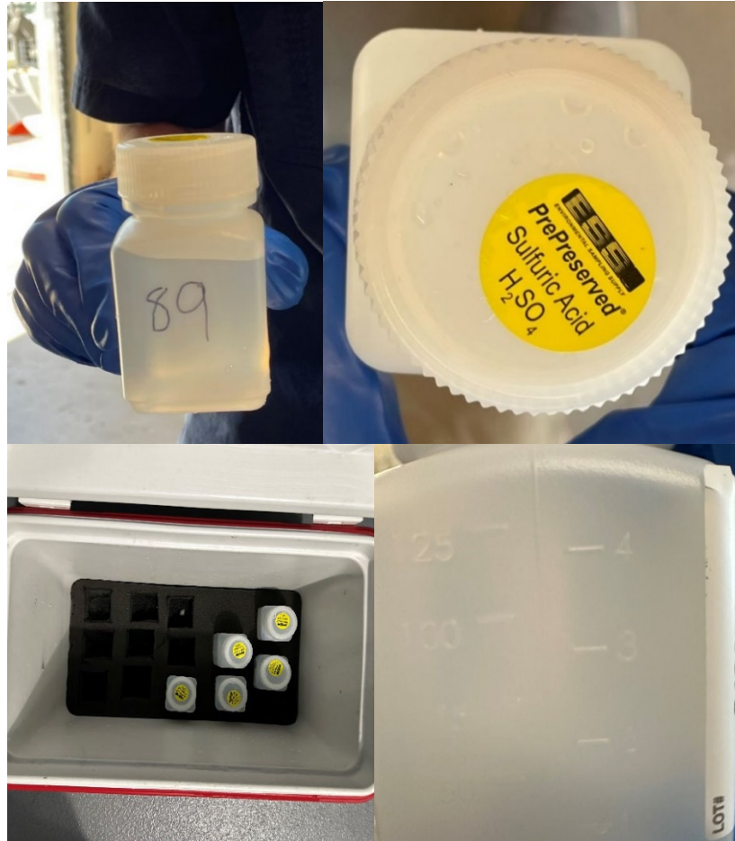
Figure 2: Pre-preserved nitrate sample bottle, ice chest containing pre-preserved nitrate sample bottles in foam insert, and fill lines marked on a pre-preserved nitrate sample bottle.
