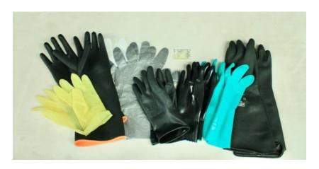
Chemical-resistant gloves must be made from one of the following materials: laminate, butyl, nitrile, neoprene, natural rubber, polyethylene, PVC, or Viton™. These materials must have a thickness of 14 mils except for gloves made from polyethylene and laminate.
