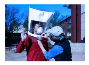
This test takes about 15 minutes to complete and is performed using the same size, make, and model of respirator that will be used by the handler on a regular basis.
