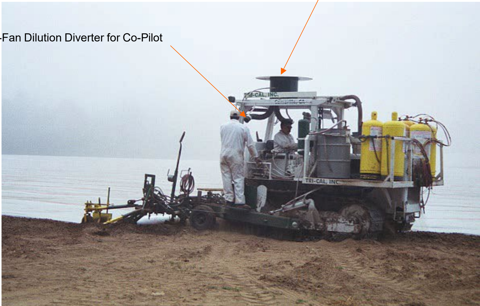
FIGURE 8. AIR-FAN DILUTION SYSTEM (TRACTOR MOUNTED/SIDE VIEW)
