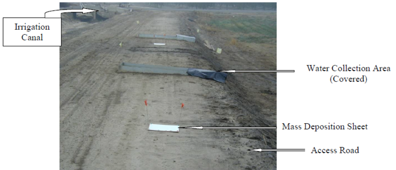
Figure 3. Location of mass deposition sheets to measure application rate of diuron. Two plots were constructed where the second plot was used as a backup.
