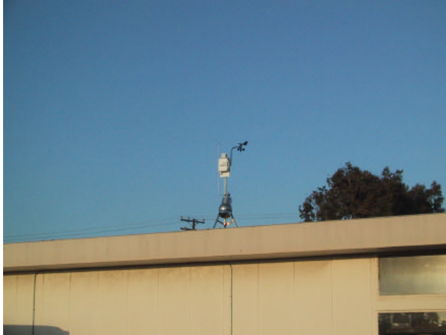
Figure 4. Sampler and micromet set up at SHA rooftop site.
