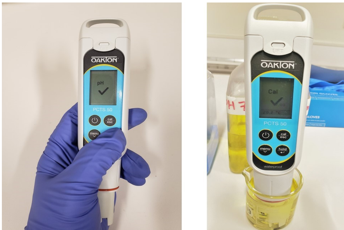
Figure 2. Left: PCTSTestr 50 pH meter displaying pH mode is selected. Right: PCTSTestr 50 pH meter submerged in a beaker with a pH buffer.
