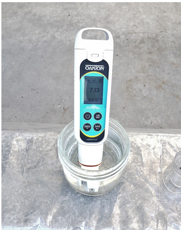
Figure 3. pH meter submerged in half-pint glass jar filled with a groundwater sample. Jar is placed on a plastic sheet to prevent contamination of equipment.
