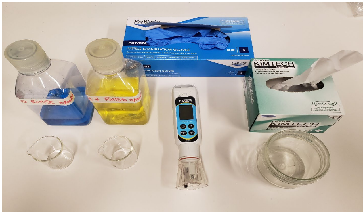
Figure 1. Materials used to calibrate pH meter: 10.0 buffer solution, 7.0 buffer solution, 2 beakers, gloves, PCTSTestr 50 pH meter, laboratory wipes, half-pint glass jar, and deionized water in squirt bottle (not shown).
