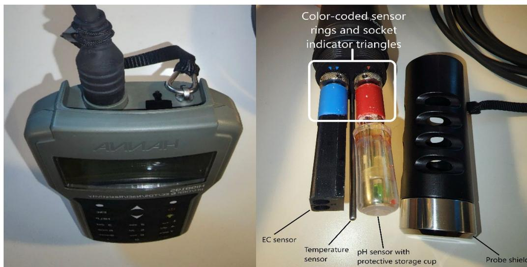
**Figure 2.** Left: Handheld meter with probe plug inserted into the device input socket. Right: Probe with probe shield removed exposing color-coded sensors and pH sensor protective storage cup.
