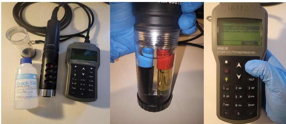
**Figure 4.** Left: Meter, calibration beaker, and quick-calibration solution. Middle: Probe with attached calibration beaker filled with quick-calibration solution. Right: Meter displaying quick calibration selected from the menu.
