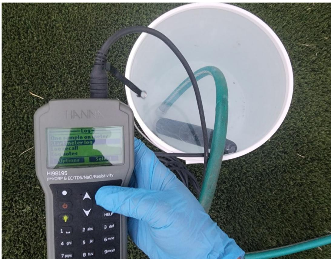
*Figure 5. Probe in 5-gallon bucket with garden hose purging a well.*
