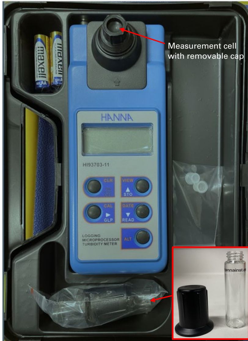
Figure 1: Turbidity meter in open case. Inset picture shows cuvette and its cap.
