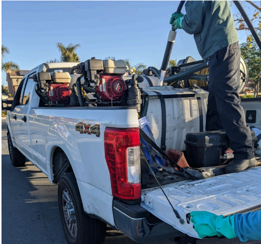
Figure 2. Applicator circulating the mixture by directing spray back into the tank.
