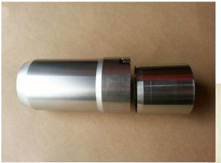
When inserting soil sample collection ring into sampler head, make sure beveled end is facing towards the sampler head's end
