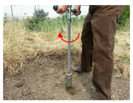
**3.10** Remove the soil sample collection ring from the sampler head.
