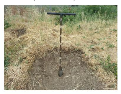
3.6 Place the fully assembled soil sampler on top of the soil sample to be collected. Drive the soil sampler into the soil to a depth that ensures the sample ring is full of soil (greater than 5cm, but less than 10cm).
