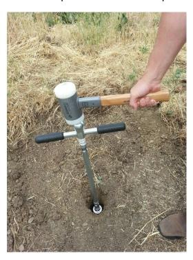
3.8 Once reaching the proper depth, turn the handle of the soil sampler 90° to break the soil at the base of the sampler from the soil below.
