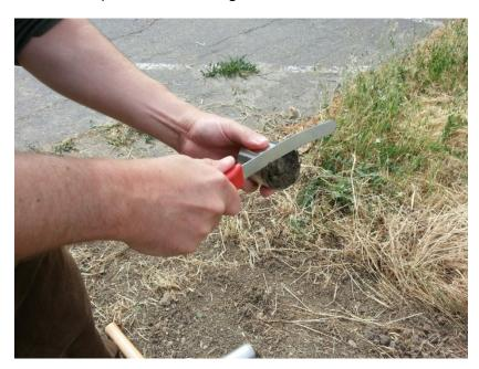
**3.12** Place caps on both ends of the sample collection ring to maintain sample integrity.
