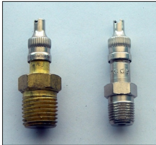
Figure 18. 1/4 inch and 1/8 inch (also called brass and silver) Schrader valves. The 1/4 inch Schrader valve may also have a chrome finish. Caps may be used to tighten or remove the valve cores. Use a 7/16 inch wrench on the 1/4 inch valve and a 5/16 inch wrench on the 1/8 inch valve.
