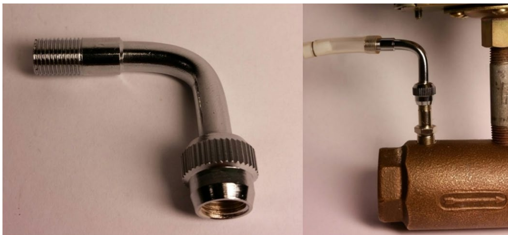
Figure 19. Left: A 90 degree adaptor. Right: A Tygon/Teflon sampling tube attached to a 90 degree adaptor that has been screwed onto a Schrader valve.
