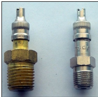
Figure 18. 1/4 inch and 1/8 inch (also called brass and silver) Schrader valves. The 1/4 inch Schrader valve may also have a chrome finish. Caps may be used to tighten or remove the valve cores. Use a 7/16 inch wrench on the 1/4 inch valve and a 5/16 inch wrench on the 1/8 inch valve.
