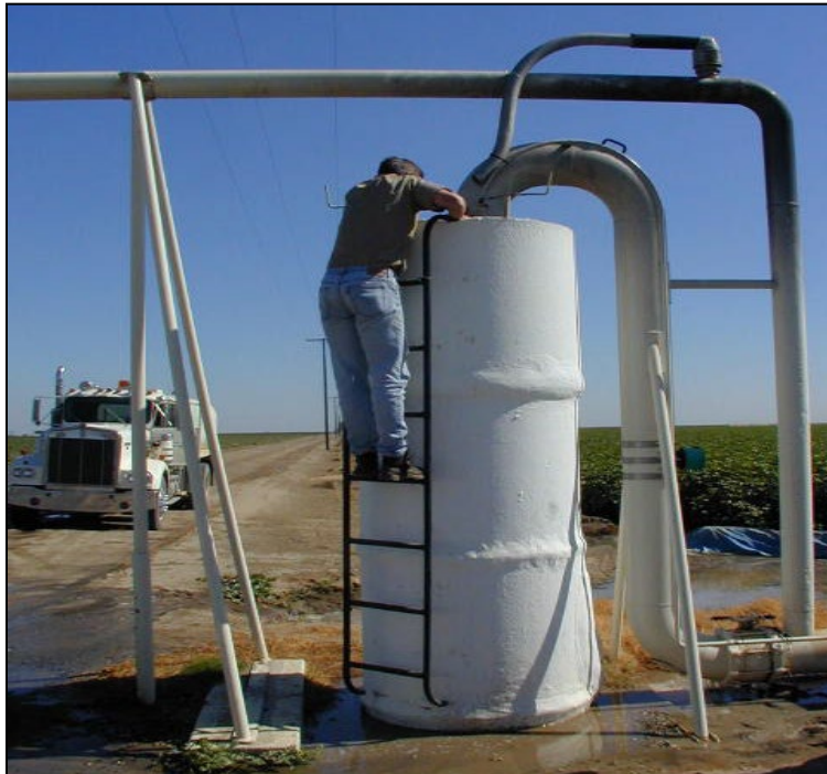
Figure 16. Sampling from a well discharge pipe into a standpipe. Extreme care is required to prevent dropping a bottle while sampling. The force of the water exiting the discharge pipe can be very high.
