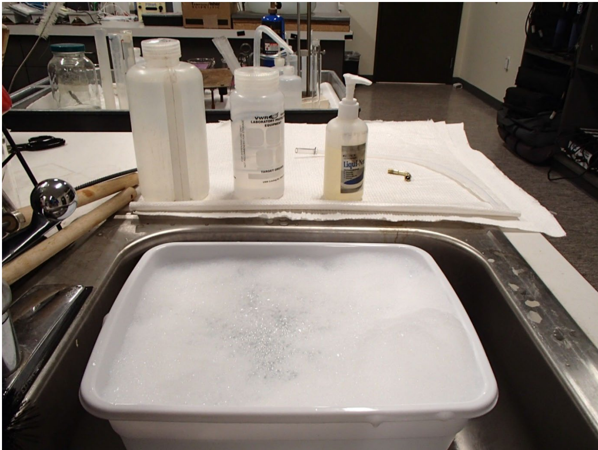
Figure 1: Example of the dishpan used to submerge equipment in a detergent solution. Pictured from left to right are DI water, isopropyl alcohol, and Liquinox® wash bottles. A 90-degree Schrader adaptor and a piece of sample collection tubing are displayed to the right of the wash bottles.
