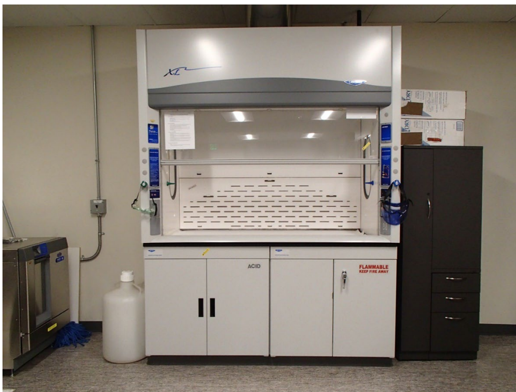
Figure 2: The fume hood used to store alcohol waste rinsate. The waste bottle will be in the solvent storage cabinet (bottom right).
