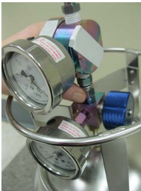
Figure 1. Mechanical regulator properly seated on Summa canister.
