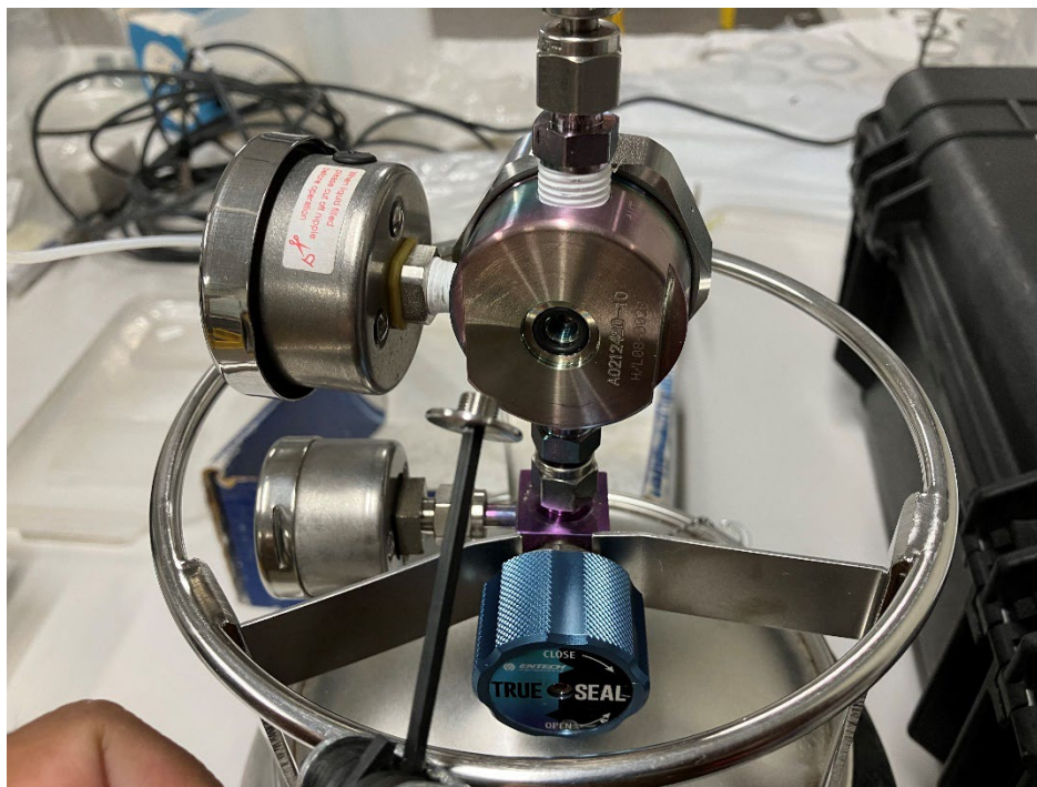
Figure 6. Flow controller with dust cover removed to expose piston gap screw.
