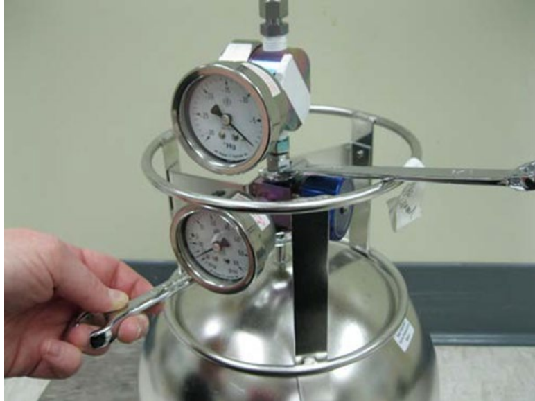
Figure 2. Proper technique to use when tightening the regulator onto the Summa canister.
