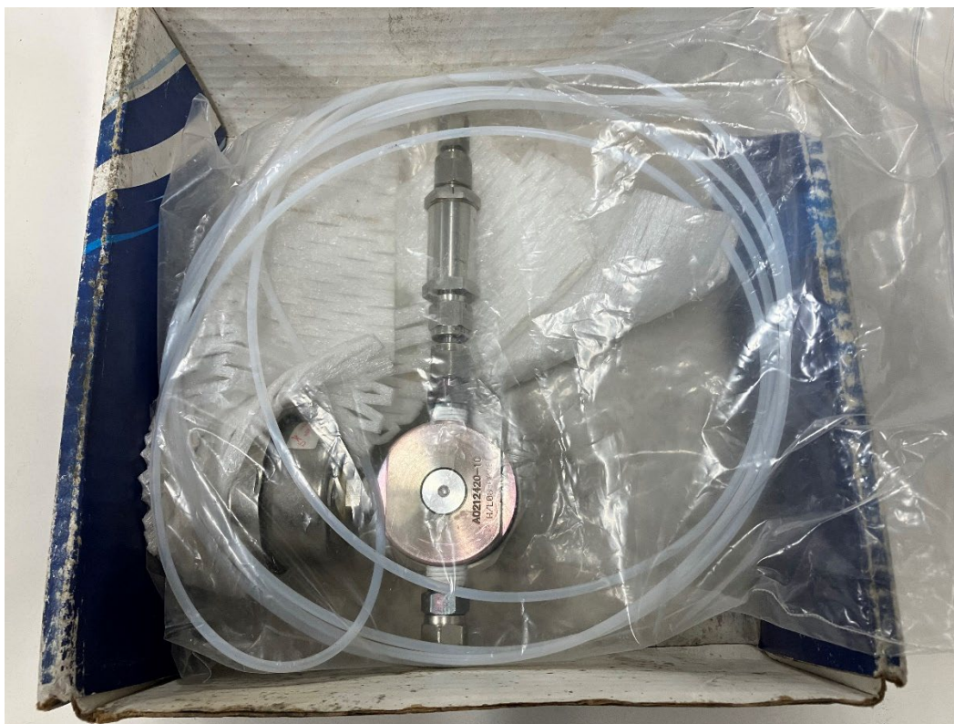
Figure 4. Properly stored mechanical regulator
