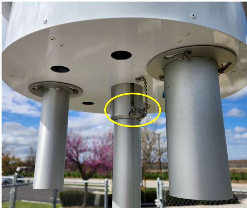
Figure 5: Location of the pin on the solar radiation shield.
