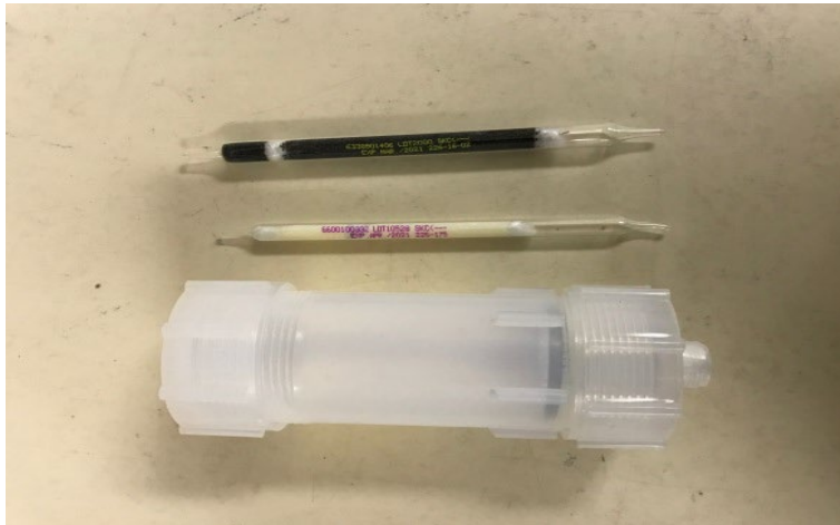
Figure 6: MITC sorbent tube (top), chloropicrin sorbent tube (middle), and multi-residue cartridge (bottom).
