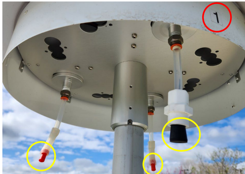
Figure 9: Plastic caps on the opening of the tubes from the last sampling.
