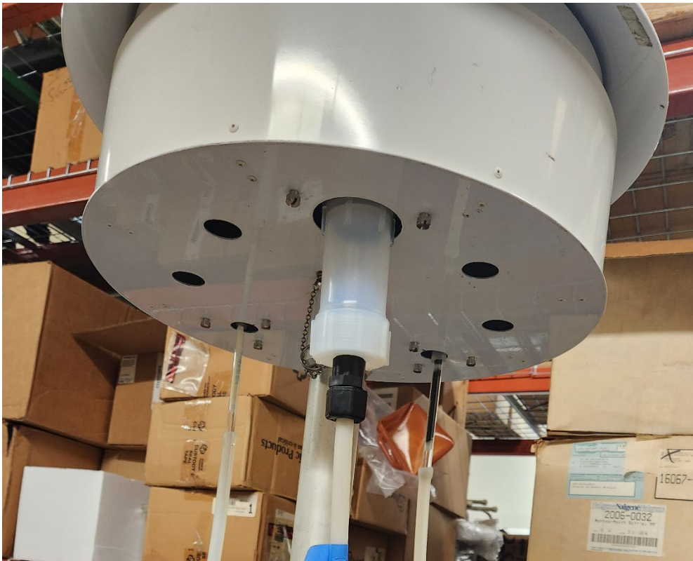
Figure 15: Proper sampling media and calibration tubing attachments to the Met-One Channel Pesticide Sampler.
