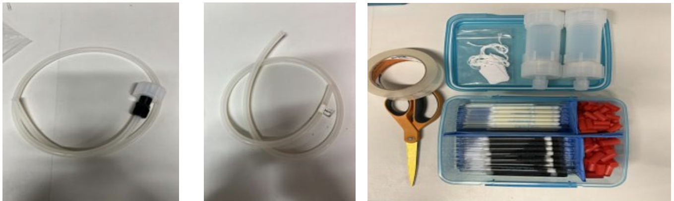
Figure 4: Connector for Multi-Residue (left picture), the connector for MITC and Chloropicrin Sorbent Tubes (middle picture), and, labels, sorbent tubes, and caps (right picture).
