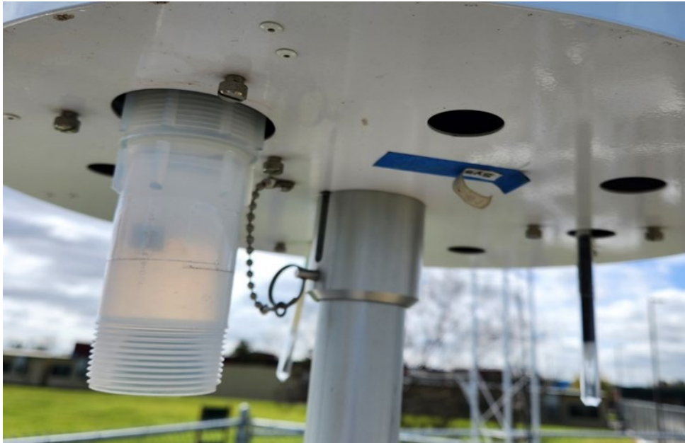
Figure 11: Solar shield in place with sample covers removed.
