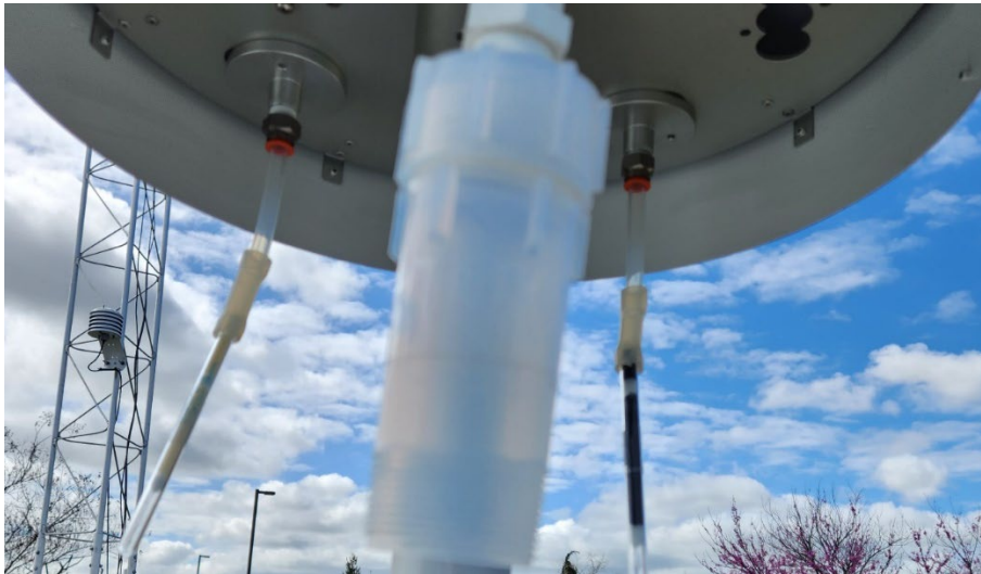
Figure 10: correct installation of sampling cartridges on Met-One
