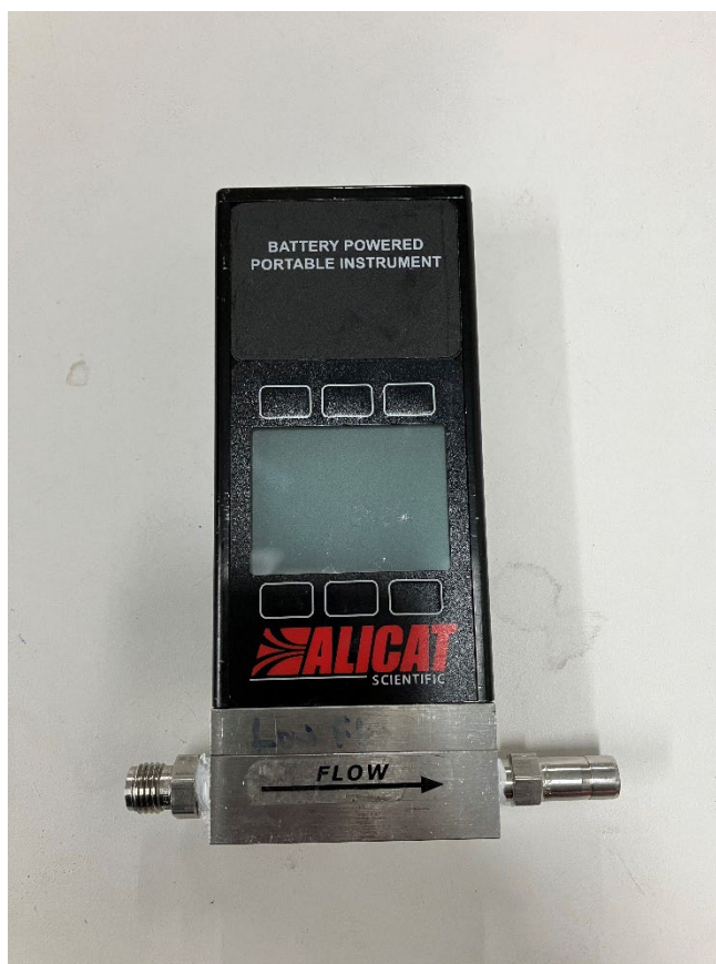
Figure 3. Alicat flow meter before being powered on. Pressing the button on the top of the device will power it on. Pressing the Alicat logo will turn on the screen's backlight.
