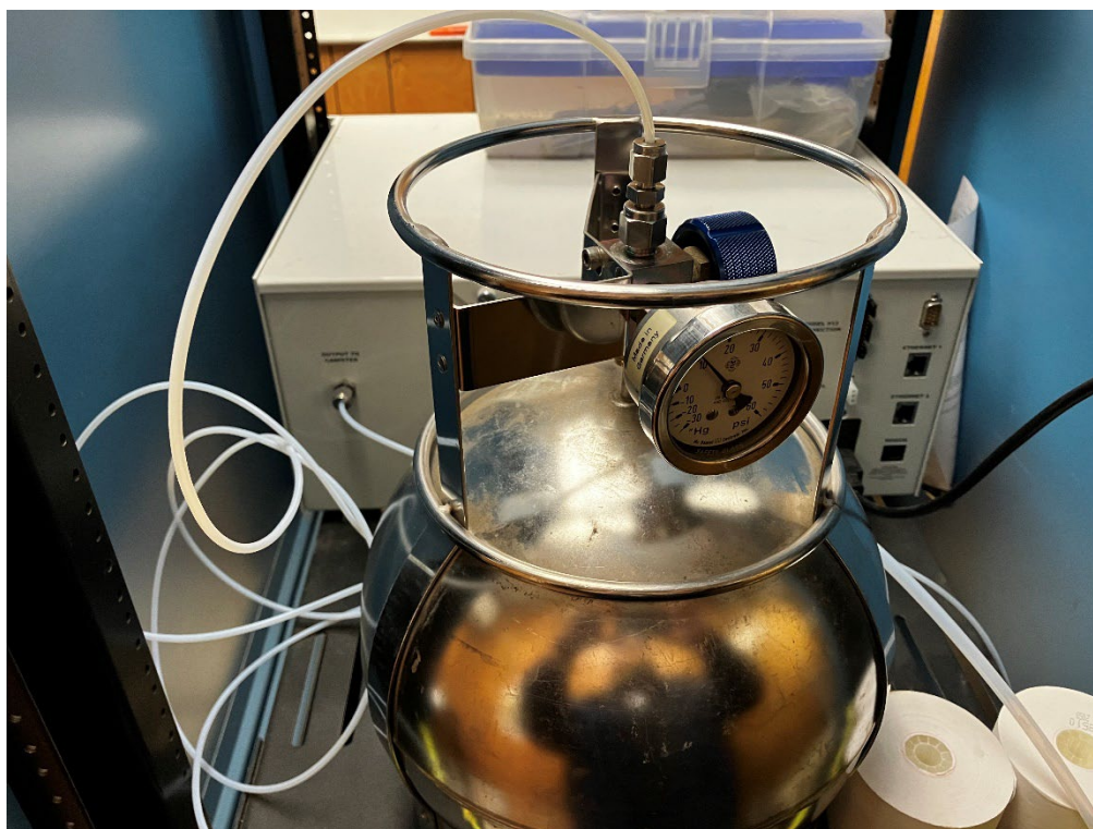
Figure 8. Xonteck 901 setup in sampling configuration. The Output to Canister port is fitted with the 'Output to Canister' line connected to a 6-L SilcoCan. Sample intake tubing leads out from the Sample Intake port and up to the sampling probe.
