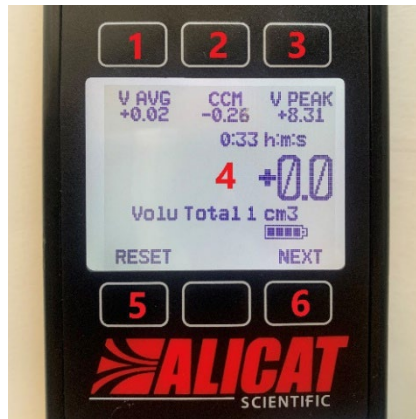
Figure 5. Totalized flow data
