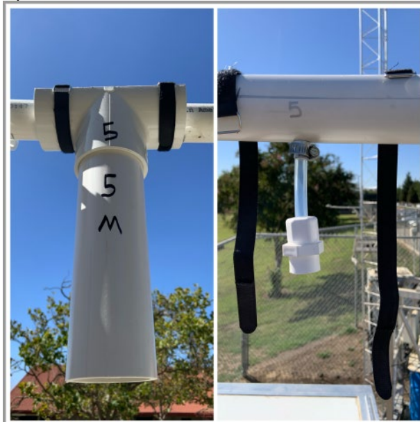
Figure 4: Removing the radiation shield cover.
