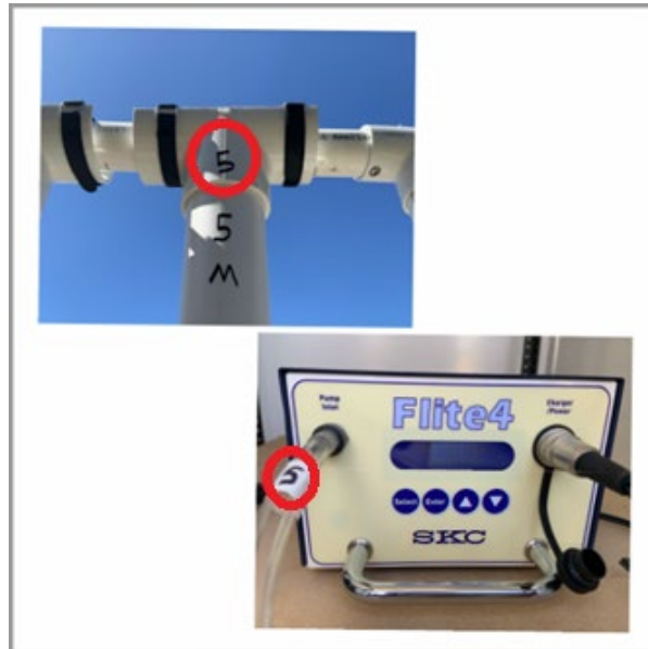
Figure 3: Identifying which sampling port to use.
