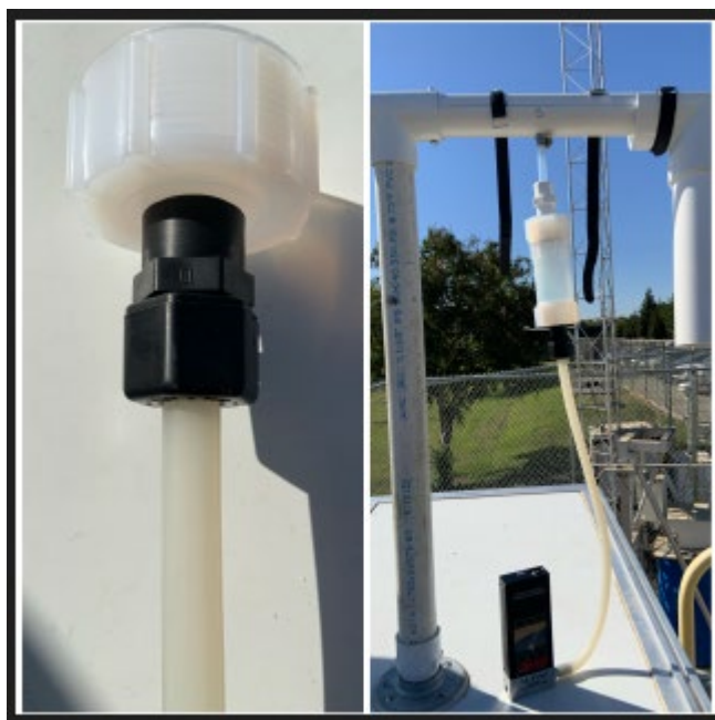
Figure 7: Connected calibration tubing.
