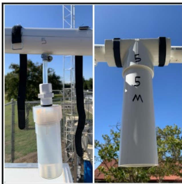
Figure 15: Solar radiation shield reattached.
