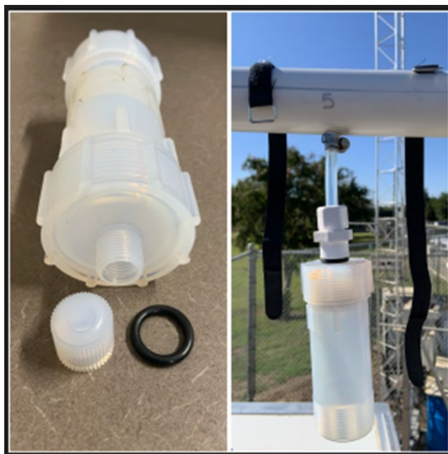
Figure 5: Multi-Res cartridge attached to the sample inlet.
