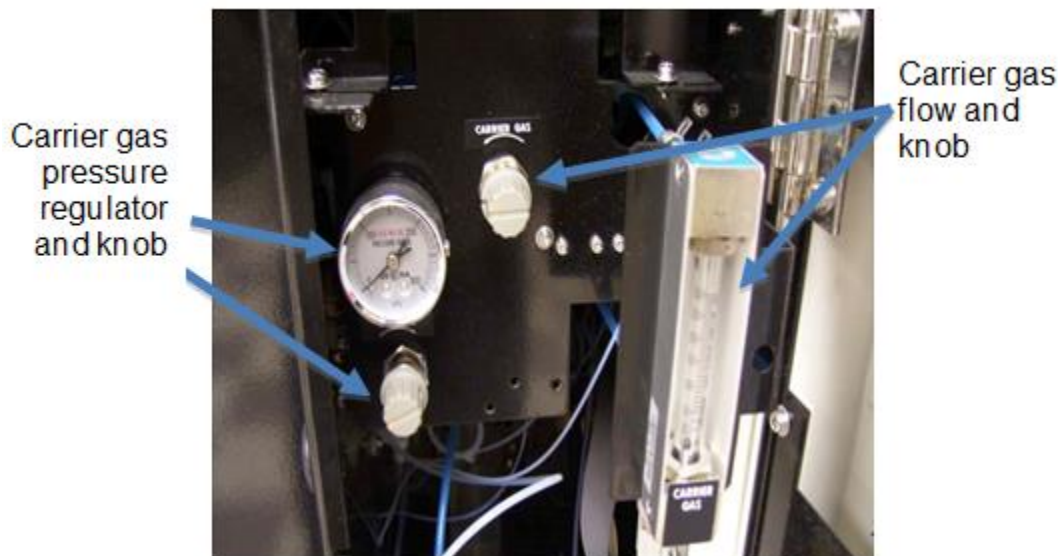
Figure 6. Setting the carrier gas pressure and flow.
