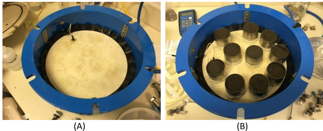
Figure 7. (A) Second ceramic plate connected to the outlet port; (B) Setup of ring samples on the second ceramic plate.
