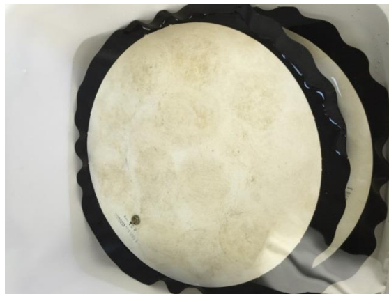
Figure 2. Two ceramic plates submerged in DI water for 24 hours.
