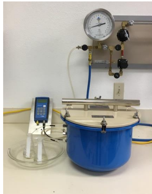
Figure 13. Two 125 mL beakers (with tape applied) used to capture and measure water.
