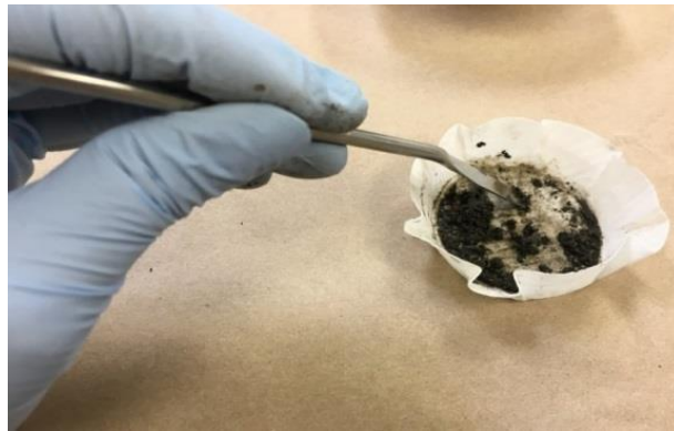
Figure 17. Cleaning soil residue from filter paper.
