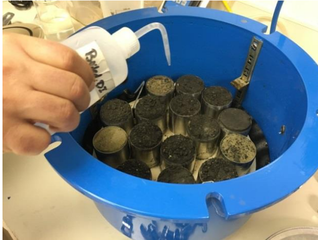
Figure 6. Additional DI water applied to the ceramic plate in between the ring samples to ensure hydraulic continuity.
