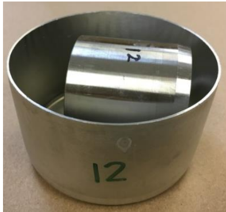
Figure 19. The soil ring sample in an aluminum can is ready to go in the drying oven.
