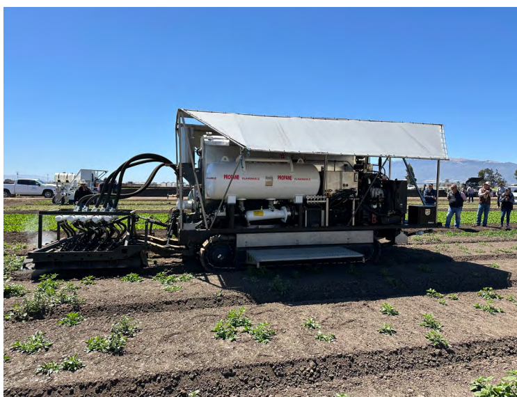
Figure 2.2. Mobile steam applicator used for soil disinfestation treatment, designed to deliver high-temperature steam (65 - 70°C or 149 - 158°F) for pest and pathogen control in agricultural fields. Photo: Jenny Broome.
